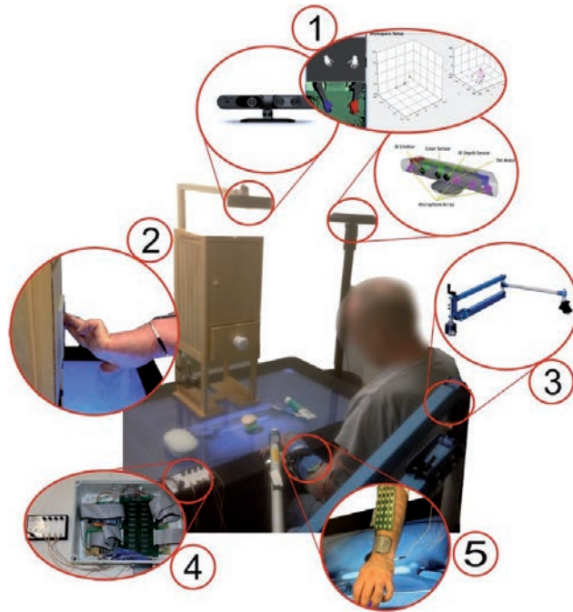
Fig. 1. The components of the GO-SAIL system: (1) Microsoft Kinect® and Primesense sensors which provide kinematic data for the ILC algorithm; (2) virtual and real tasks displayed using touch table; (3) SaeboMAS® arm support; (4) FES and multiplexor hardware (5) surface electrode array on forearm.
